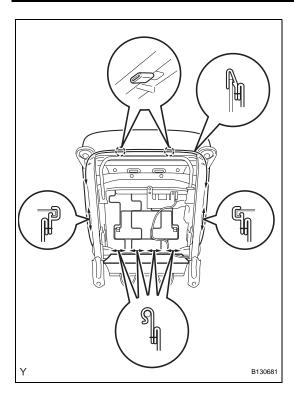
(c) Disengage the 2 claws and the 7 hooks and remove the front seat cushion.
