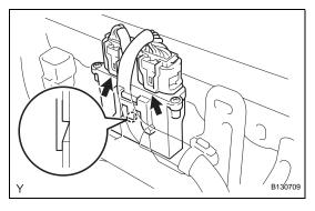
(b) Using a screwdriver, disengage the claw and remove the occupant classification ECU.
